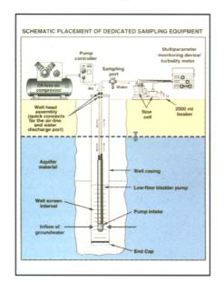
During sampling, groundwater is discharged to an in-line flow cell that measures pH, specific conductance, redox potential, temperature, dissolved oxy-
