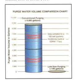
Low-flow purging also reduces the time spent to purge and dispose of water. Compared to conventional methods using dedicated equipment, two to four hours of time were saved at each well deeper than 50 feet. When compared to the use of portable non-dedicated equipment (which can operate at higher flow rates), only five to 15 minutes were saved at each well. However, this did not reflect the time spent decontaminating equipment between wells and collecting equipment rinsate blanks to
