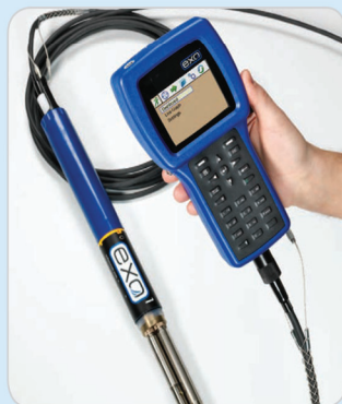
Interface with the EXO Sonde using the EXO Handheld Display
