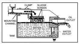
along with the oil. When used in tandem with the oil skimmer, an Oil Concentrator will solve this problem, and provides virtually complete oil /water separation, saving money and improving the efficiency of the skimmer.
