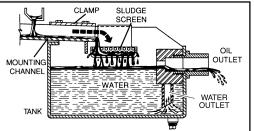
along with the oil. When used in tandem with the oil skimmer, an Oil Concentrator will solve this problem, and provides virtually complete oil /water separation, saving money and improving the efficiency of the skimmer.
