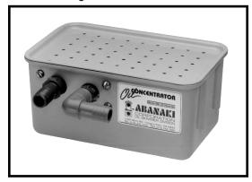
Decanters save money and improve efficiency by almost completely separating any coolant from the skimmed tramp oils. Oil-free coolant discharged from the decanter is returned to the original tank or directed to a separate container. Virtually no costly coolant gets thrown out
