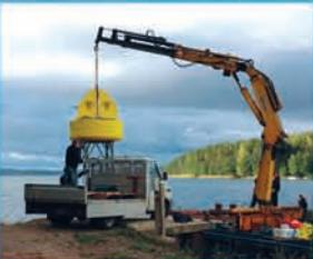
**Source water management** customers use our automated vertical profiling systems to target treatment processes and reduce the cost of operations.
